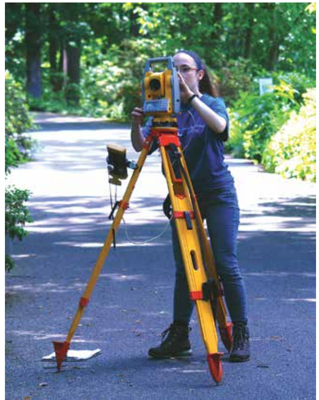
Fig. 14. Using the Total Station to map plants in the field.
